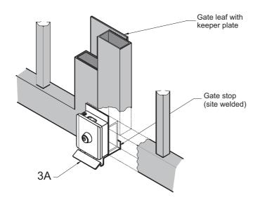
The swivel dead bolt of the FAAC electric gate lock (400504) and the Viro V90 electric gate lock (400505) are designed for locking automatic and manual gates.
