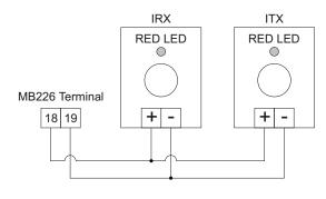
Red LED constant ON = PE aligned Red LED flashing = PE unaligned
