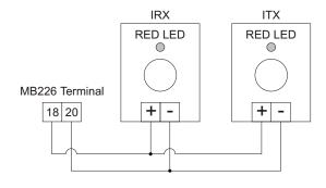
Red LED constant ON = PE aligned Red LED flashing = PE unaligned
